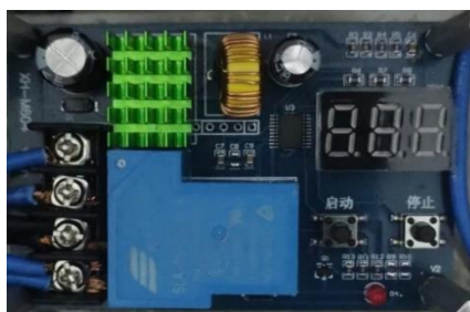
Gambar 5. High Voltage Disconnect (HVD)
