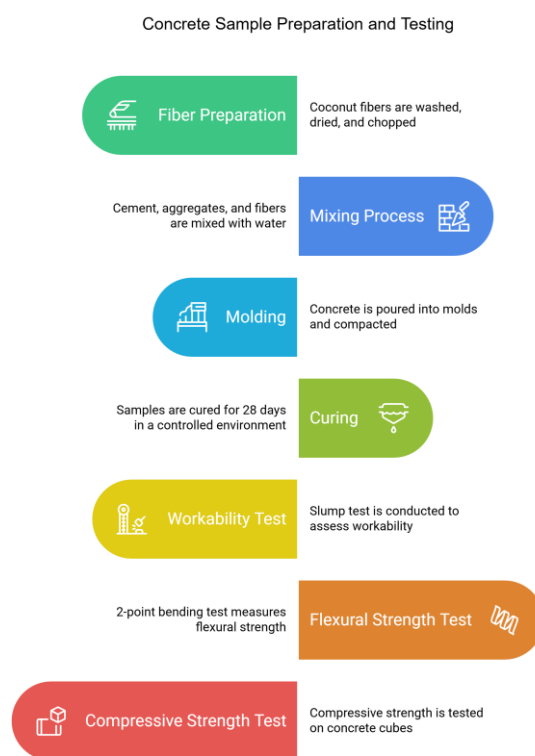
Figure 1. Flowchart Concrete Sample Preparation and Testing Process
